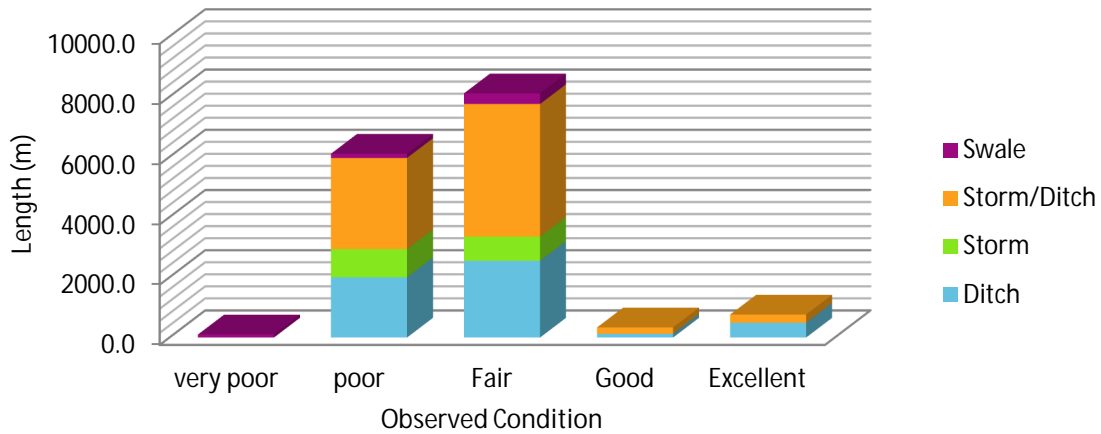
Figure 2.2-2: Drainage Assets Condition
